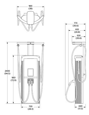
Express Plus Power Link 2000, with non-liquid cooled cables, single connector
