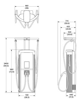
Express Plus Power Link 2000, with liquid cooled cable, single connector
